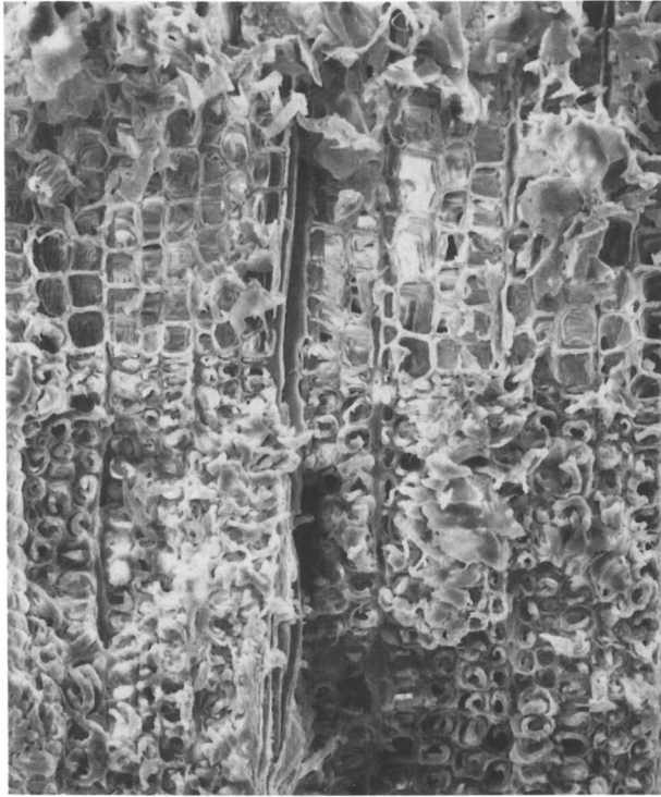
Figure 13. Scanning electron micrograph of transverse section of air-dried Picea sp. from a 1200 A.D. Thule site, Herschel Island. The fractured surface shows oil-swollen secondary cell walls of latewood tracheids separated from the primary wall complex. This is shown in detail in Figure 14. The earlywood tracheids appear normal.
