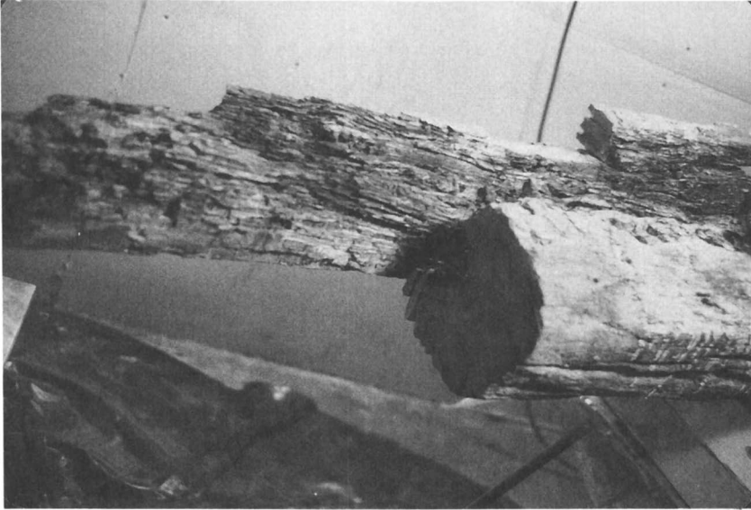
Figure 17. Upper section of post illustrating insect and fungal degradation. Large cut section resulted from section being removed for sample taken aboard spacecraft Endeavor .
