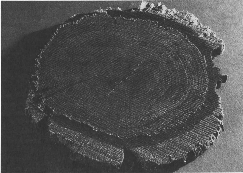
Figure 2. Oak with a central portion of "woolly" appearance surrounded by clean-cut highly degraded heartwood and sapwood.
